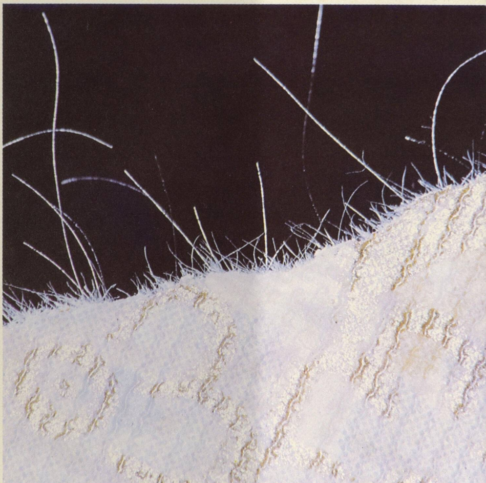
Polyester plastic fibres act as a strengthening agent in Tonecraft's dry-strippable wallpaper. (Photo: Bruce Kane, NRC)
