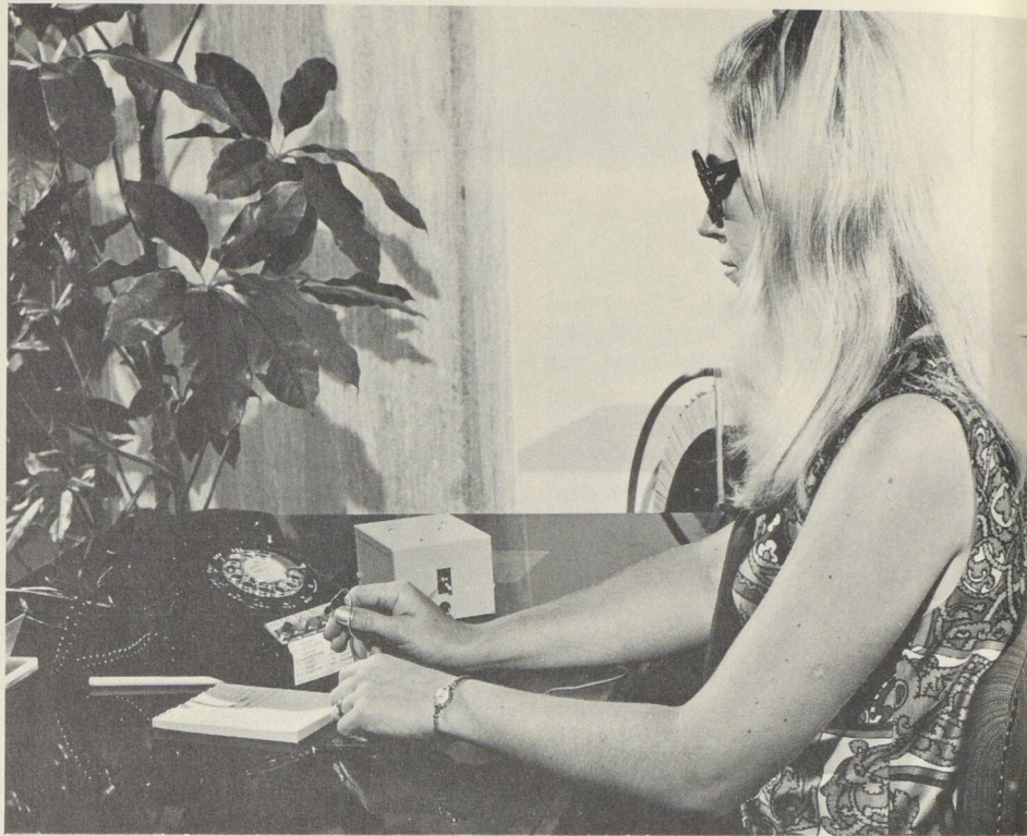
Light detector enables blind switchboard operator to locate flashing light indicating an incoming telephone call.
