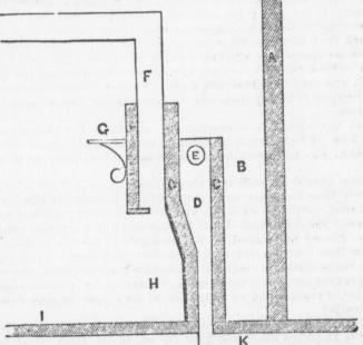
H Fireplace. B Space between Hot Chamber and Wall. C Brick Walls 4 inches thick. D Hot Air Chamber. E Opening for the escape or shutting off Hot Air. K Air Box for the supply of fresh air, extending beneath the floor to the front door. F Iron Smokeflue S inches diameter. G Front of the Fire-place and Mautle-piece. I Solid Hearth. The above Plan has many advantages. It secures a more equable diffusion of heat,
