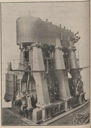
gines, with cylinders 28 inches, 46 inches and 77 inches in diameter, respectively, for the high, intermediate and low pressure, has a stroke of 54 inches, and the all-round reversing gear and the turning gear are operated by independent engines.
