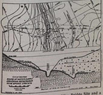
Location of the Ashokan Dam at Olive Bridge Site and a Geological Cross-section
