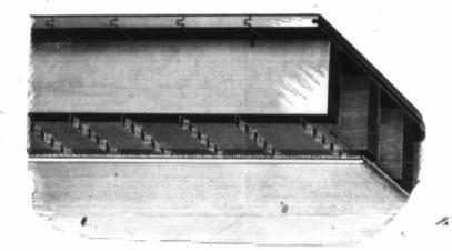
This lathing consists of a combination of wire cloth, 3% in mesh, made of No. 18 steel wire, and a crimped iron furring varying from 3% to 1 in. wide. In applying, the furring strips are first stapled across the joists every nine inches, the cloth being then stretched over and stapled and tied to the furring giving great strength and stiffness to the fabric.
