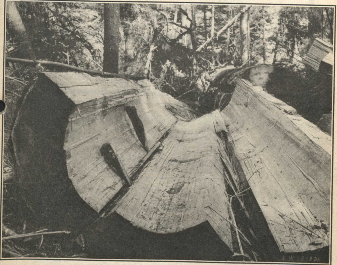
SHOWING HOW A BRITISH COLUMBIA SPRUCE LOG IS "RIVED" IN PREPARATION FOR AEROPLANE MANUFACTURE. (PICTURE BY COURTESY "THE LUMBERMAN.")
