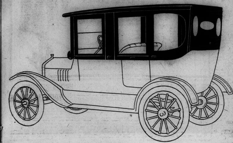
The deck is of No. 1 ash and poplar, ribbed crosswise, curved and statted endwise. The slats being counter-sunk, all joints and laps are glued, screwed and nailed. The roof covering is in one piece, and of double texture two-ply sail duck, with rubber between. No seams to tear, rot or leak. The exposed side is heavy rubber-coated and grained, semi-bright finish.
