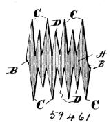
four rows of points are formed, the projections at one edge staggered with relation to those at the opposite edge, so that each projection is arranged opposite and pulls against a long and short projection, the four corners of the fastener having the long projections, substantially as described.
