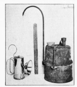
two serious faults. The smoke from it is often so great as to drive men two serious faults. The smoke from it is often so great as to drive flet out of small workings, many mines requiring extra ventilation on this account. In gold and silver mines it cannot be used successfully because spilled oil interferes with the separation of the metal. From what figures are obtainable the cost of this method seems to average about 5 cents per miner's lamp for eight hours use.
