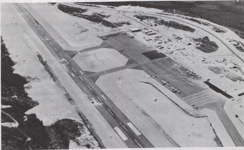
The first airstrip, La Grande Airport, was opened in 1973; it was built by widening an existing dirt road. The airport, the largest of five built to serve the complex, services LG2 and LG1. Two commercial airlines provide daily flights from the airport.
