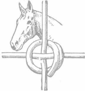
and strand wires cross. This tremendous direct pressure bruises and injures the wires—this is quite apparent if you remove the lock, and is sufficient to make the wires an easy prey to frost, snow or heavy strains.
