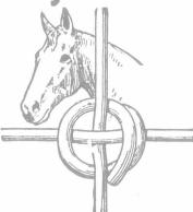
and strand wires cross. This tremendous direct pressure bruises and injures the wires—this is quite apparent if you remove the lock, and is sufficient to make the wires an easy prey to frost, snow or heavy strains.
