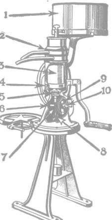
Worm wheel clutch stops all mechanism when crank is stopped, with exception of bowl and worm wheel. No lost motion in again starting crank as clutch grips instantly and without jar to the mechanism.
