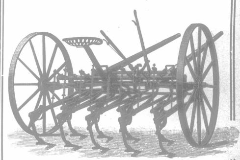
THE CLIMAX cuts to a depth of 2 or 10 inches and leaves a compact seed-bed while loosening the surface soil to retain the moisture.
