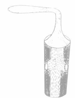
Fig. 3 Showing drilling of three way stopcock
