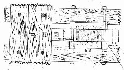
This illustration represents a set of No. 68 Butler Drawbar Attachments, applied as we recommend. We show an 1x4 inch wrought strap or yoke, a less size can be used if desired. Yoke cannot get out of place on account of side walls. No bolt through center necessary to hold springs in position.
