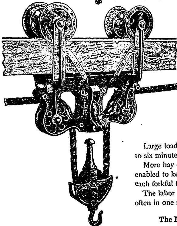
The *Carrier* is a truck having four wheels with a broad tread, running upon a wood track suspended from the rafters of the building, by means of which the fork with its load is drawn directly up to the highest point of the building, and is then carried off over the mow, clearing the mow and all beams, ties, etc., that interfere with other modes of using horse forks.
