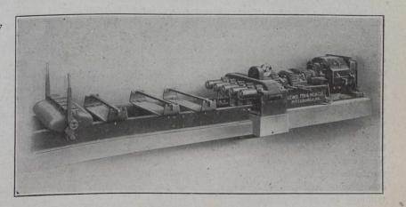
the twisting process, which usually results in an inferior product due to the elastic limit of the bar being exceeded. With a motor gear-connected to the machine, as shown in the accompanying illustration, an occurrence of this kind is practically impossible, since this method of motor connection insures constant torque being applied during the time the bars are being twisted.
