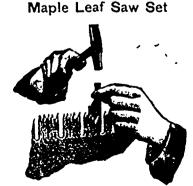
otions.—Place the Set on the point of tooth as shown in the above cut, and strike a very light blow thammer. If you require more set, file the tooth with more bevel. If you follow directions you can mistake. Be sure and not strike too hard a blow, and it will set the hardest saw.
