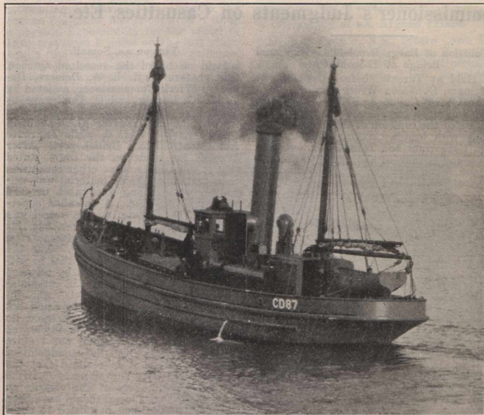
Wooden steam drifter, built by Canadian Vickers, Limited.
