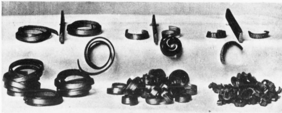
Fig. 2. Samples of Chips and Cutters: Cutting Angles from Left to Right 45 Deg., 60 Deg. and 75 Deg. These Chips were Produced in an Engine Lathe with Holder Shown in Fig. 12. The Chips were Confined Edgewise Between the Body of Work and the End of the Holder. The Breakage of Chips Taken by the 45 Deg. Tool were due to Chips Getting Caught Between the Work and Tool Holder, Usually due to the Irregular Winding of the Chip. The Chips Produced by the 60 Deg. Tool Wound up till the Circle was Greater than the Chip Could Take Without Breakage.
