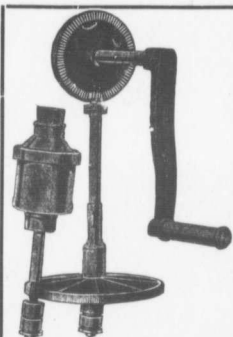
Showing extreme simplicity of driving gears—one pair bevel gears, one pair spur gears, showing also the inclined intermediate shaft, a new and exclusive "Simplex" feature.
