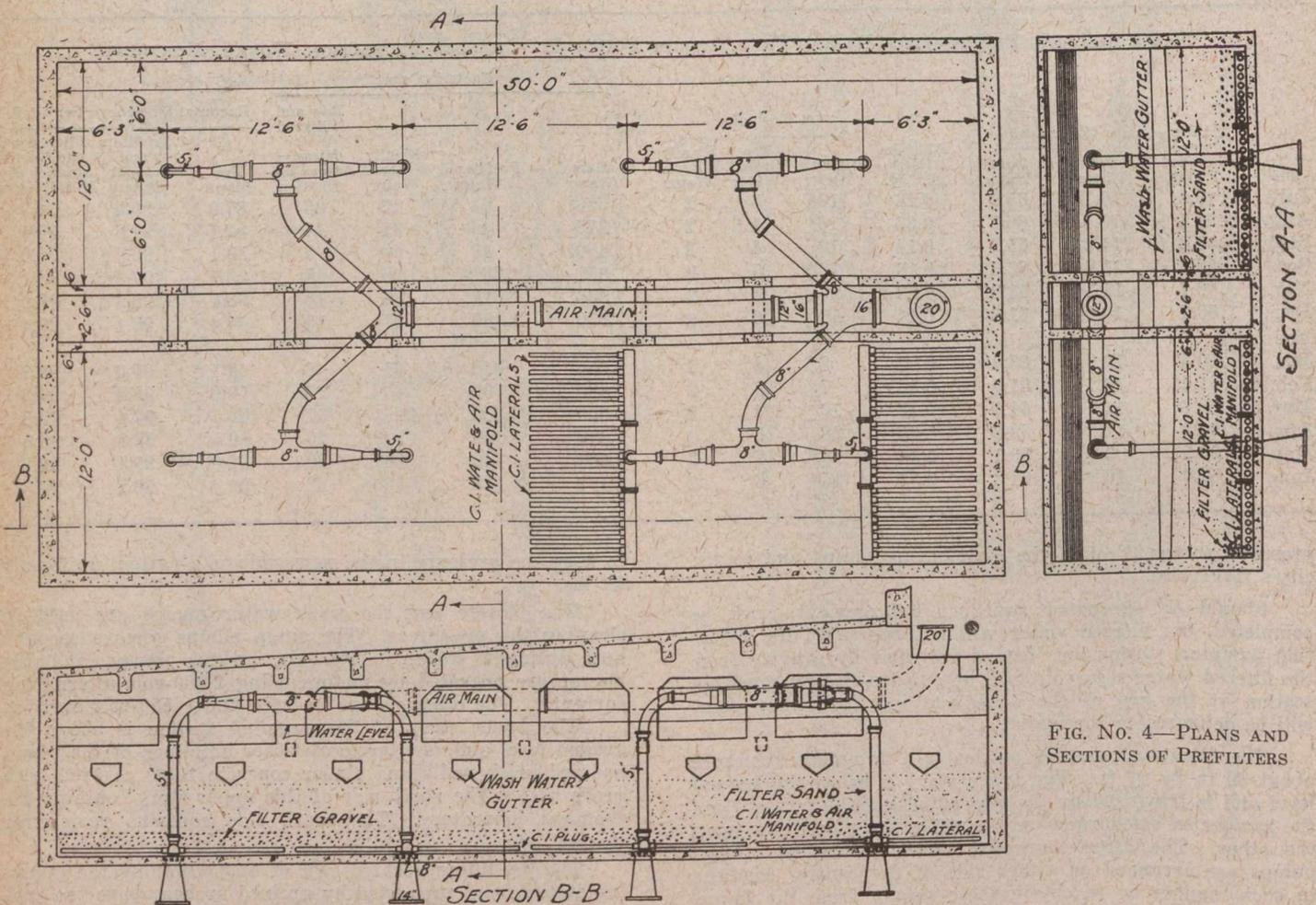
FIG. NO. 4—PLANS AND SECTIONS OF PREFILTERS
