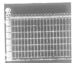
The uprights or pickets are all made of the best No. 9 hard, galvanized wire, and are 3 ins. apart, The line wires are two No. 12 wires, twisted.
