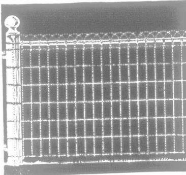
The uprights or pickets are all made of the best No. 9 hard, galvanized wire, and are 3 ins. apart. The line wires are two No. 12 wires, twisted.
