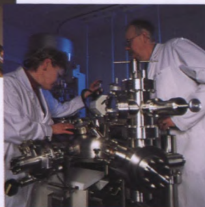
Specimen undergoing X-Ray Photoelectron Spectroscopy (XPS).
