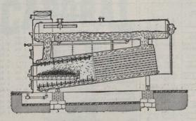
An externally fired boiler wastes fuel because of the radiation of heat from the outside of the brickwork and the leakage of cold air above the fire, which causes a double loss by heating the excess of air and by producing imperfect combustion.
