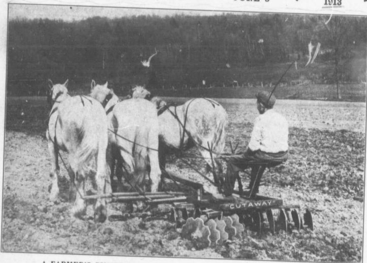
A FARMER'S BUSINESS ABILITY IS REFLECTED IN HIS IMPLEMENTS The Double Cutaway Harrow, here illustrated, enables a man to do in one day as much work as he formerly did in two with the ordinary disk harrow. The same is true of the gang plow, the two row cultivator, the corn binder, and so on all along the line of improved farm implements. Why then complain of high wages for labor. If wages have increased, opportunities for employing that labor profitably have increased in even greater proportion. The business-like farmer, by using implements that are efficient and up-to-date, employs high-priced labor to his own and the laborer's advantage.
