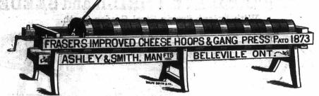
Warranted Capacity of Resisting from 40 to 60 Tons Pressure. Hi Recommended by all Cheese Makers. Prices Reduced for 1885. Price of Hoops, exclusive of Press:—12 or 15 inches diameter, to press cheese 8 to 10 inches in height, weighing from 45 to 60 pounds, \$5.50 each.
