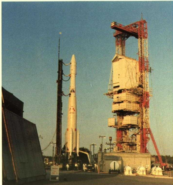
The United States provided rocket and launch facilities for the ISIS series; Canada provided the satellites. This Delta rocket was used to launch ISIS II in 1971.
