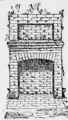
high, and has the number of courses of bricks above the opening that shown in the cut. The panel is three inches deep, and the upper course of brick in the mantel projects three inches, giving a mantel of six inches; but the design is to have a slab of red granite fitted above the projecting bricks which will project an inch over the upper
