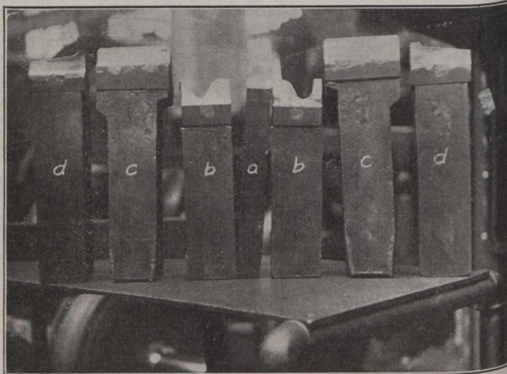
Fig. 3.—Tools for Tire Turning in Passenger Car Wheel Lathe.
