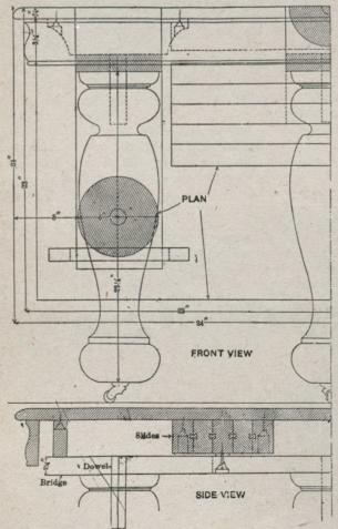
perpendicular centre line for the table. Under the top stock and 3½ inches down, draw the lower edge of rim, then 8 inches from the edge of the table draw a centre line for the leg.
