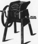
This style is very popular. It is so constructed that turnips and other roots are firmly held in place, so that there is no chance of their rolling when they come in contact with the knives. It cuts up all kinds of roots thoroughly, saves time and stock and is much more efficient than other makes.
