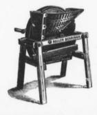
And here are two first-class machines. This one has six reversible knives for pulping and slicing. The drive wheels are large and heavy, and we use roller and ball bearings, ensuring first-class work and easy operation.
