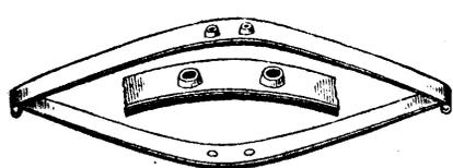
All now made with Armstrong's patent re-enforced holes (see centre of cut). These being punched without loss of stock leave the spring fully stronger than that at any other part of the plates, and being recessed into the bearing block in attaching, take away all wear or strain from the bolts, doing away with former objections to bolting, and making a very secure fastening.
