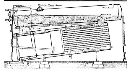
Usually built with sheet steel case, but if preferred the case may be left off and bricksetting substituted.
