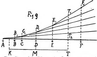
The ordinates of the different points  $B_1$   $C_1$  etc., measure the moments in relation to B, C, etc., of all the weights at the left, and if we want to find the values  $R \times N l$  and  $M_1$  when M is at D and the ends of the truss at K and  $T_1$ ,  $M_1$  will be measured by  $D_1$   $D_2$  and  $R \times N l$  by  $T_1$   $T_2$
