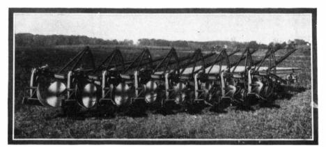
Ample strength of frame and beams. Perfect control of each plow through individual lever and large closed gauge wheel. Each plow provided with individual adjustable bracket and large swivel coulter. Guaranteed soft center shares.
