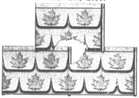
SAFE LOCK SHINGLES. This cut shows the locking device
