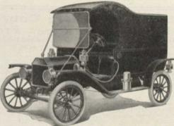
\$875 4 cylinders, the regular Vanadium Steel constructed chassis which has made the FORD Model T world famous; steel body, giving roomy interior. Capacity 750 pounds of merchandise, complete equipment as follows: Automatic Brass Wind-shield; Speedom eter; two 6-inch Gas Lamps; Generator; three Oil Lamps Horn and Tools; Ford Magneto built into the motor.
