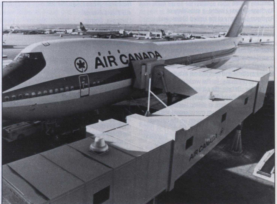
Passenger loading bridge
