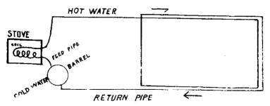
coil, and a barrel for water. The size of the greenhouse is 30 ft. by 16 ft. The pipes run under the beds. I send you ground plan of it, and will be pleased to answer through your journal, any questions concerning it.
