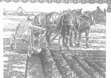
There is a spring on the land wheel which, in connection with the two bails on which the plow is hung,
