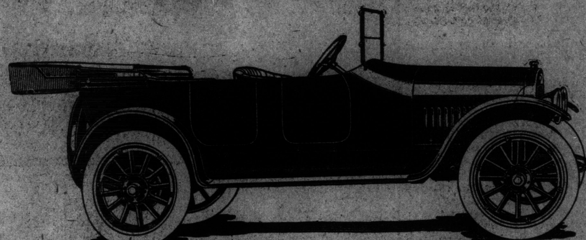
Full Elliptic Springs Front and Rear, 125-inch Wheel Base.
