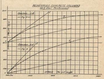
Evidently, for stresses accompanying or approaching the elastic limit of the steel, an approximate value for Ec of Es 1,000,000 may be taken. This will render n, the ratio-- equal
