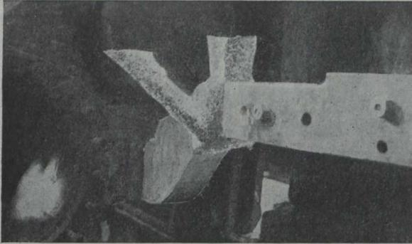
Thermit Weld on Engine Frame. Repairs of This Kind Are Made in 12 Hours or Less.
