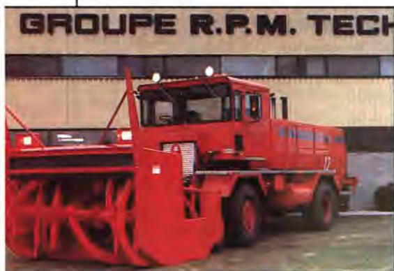
Model P-5000-R-56, two stage ribbon with over 1,000 H.P. This snowblower is high speed and will blow over 4,000 tons/hr.
