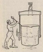
The intense heat developed by Thermit finds a very natural application in foundries for superheating and reviving dull iron in the ladle, thus improving the metal and guarding against defective castings.
