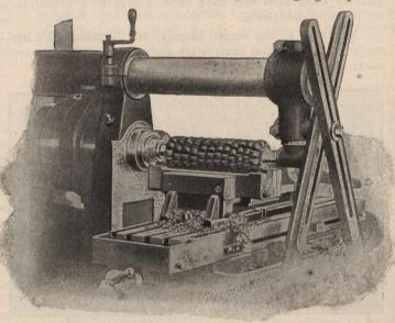
relieved cutters 31/2" diameter, forming a gang 12" wide, so that with the bars held in a vise adapted for the purpose, the entire edge of the piece is milled at a single cut.
