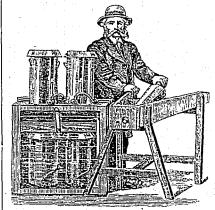
The illustration shows four tin tanks or cans, 8½ inches in diameter by 20 inches in depth, two submerged in water, and two on top, the better to show the construction. The box, or "cooler" as it is
